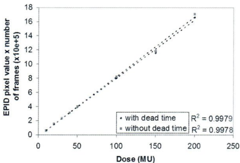
Fig.4 The response of EPID with integral dose in 10 x 10 cm 2 field size with and without dead time.
