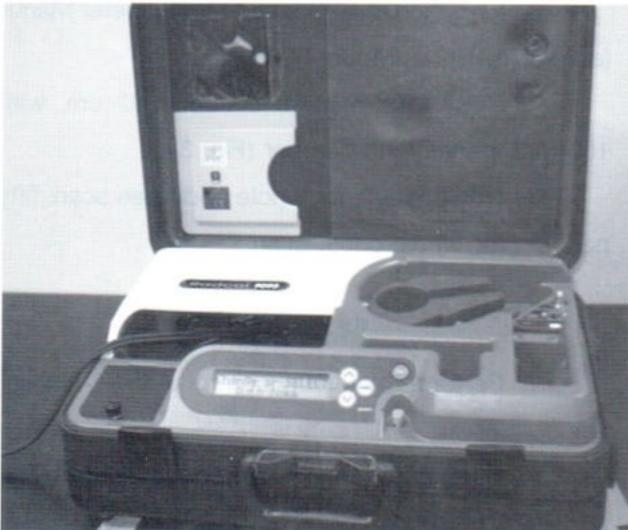
**Fig.2** Ionization chamber and Electrometer Manufacturer RADCAL Model 9095
