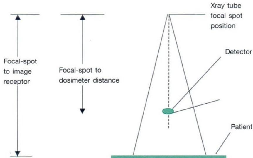
**Fig.3** Geometry used for X- ray output measurements
