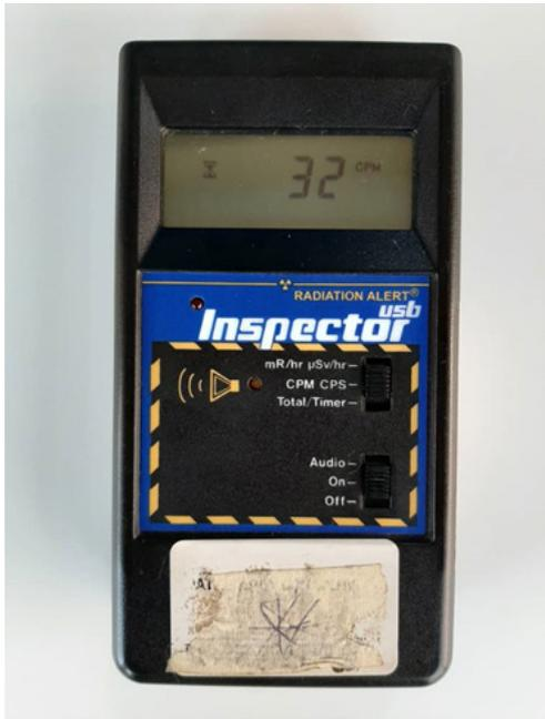
**Figure 1.** *The Inspector USB Survey meter in counts per minute (CPM).*
