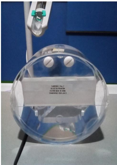
**Figure 2.** *Test phantom (Helios QA Phantom).*
