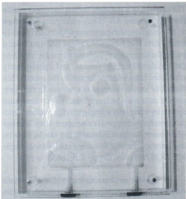
Fig.1 A hollow background chamber simulates atrium, aorta, liver and spleen
