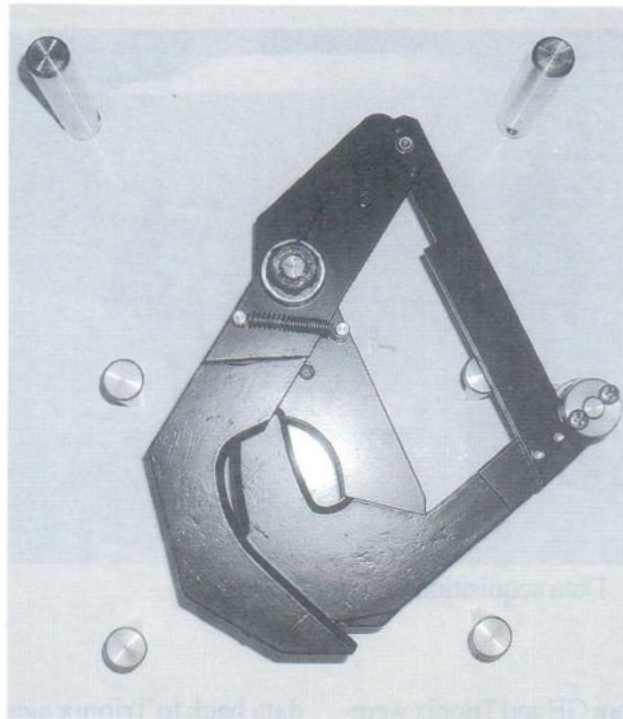
Fig.3 Metal jaws to simulate the beating heart
