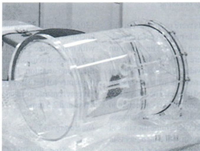
Fig. 1 Setting of NEMA NU 2-2001 phantom, inserting with hollow spheres, inserted in the water filled phantom.
